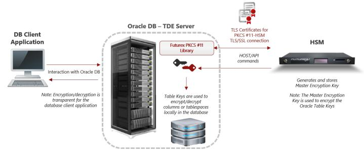
FIGURE: PROCESS OF ORACLE TDE INTEGRATION
