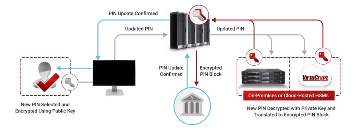
When performing a PIN change through an issuer's website or mobile app, the new PIN is encrypted using the web browser or app's RSA public key. It is then sent to the VirtuCrypt service instance. Within its FIPS 140-2 Level 3 and PCI HSM compliant boundary, the HSM translates that PIN into an encrypted symmetric PIN block and provides it in a response stored in the issuer's PIN database for future use.
